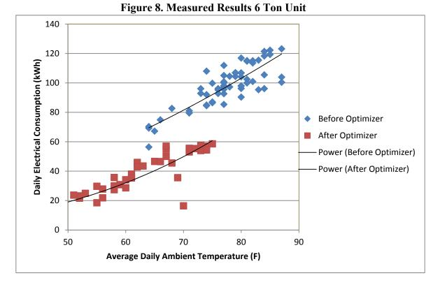
Table 3 presents the pilot results of 20 individual units. The two units with the most savings and the two units with the least savings were removed to more accurately represent the average. Measurements were made over the early winter months in order to project annual savings on a unit by unit basis. These measurements utilized American Society of Heating Refrigeration Air-conditioning Engineers (ASHRAE) bin weather data for Omaha, NE applied to the consumption curves.
