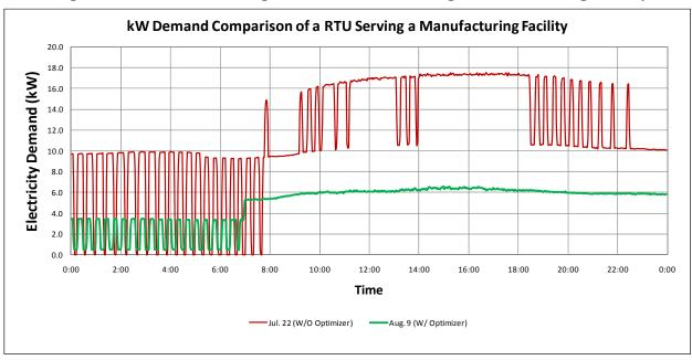
Figure 3. kW Demand Comparison of a RTU Serving a Manufacturing Facility
