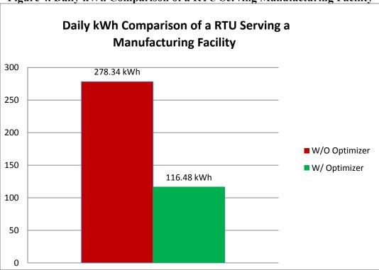
Figure 4. Daily kWh Comparison of a RTU Serving Manufacturing Facility
