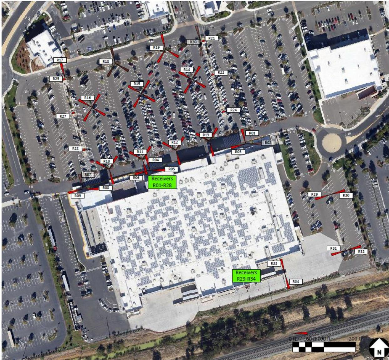
**FIGURE 28: SENSOR LAYOUT AT THE BIG BOX STORE HOST SITE IN NORTHERN CALIFORNIA. R01–R34 REPRESENT THE LOCATIONS OF SENSORS AND RECEIVERS USED AT THIS SITE. THE RED TRIANGLES EXTENDING FROM THE RECEIVER LOCATIONS REPRESENT INDIVIDUAL SENSORS AND THEIR ORIENTATIONS.**
