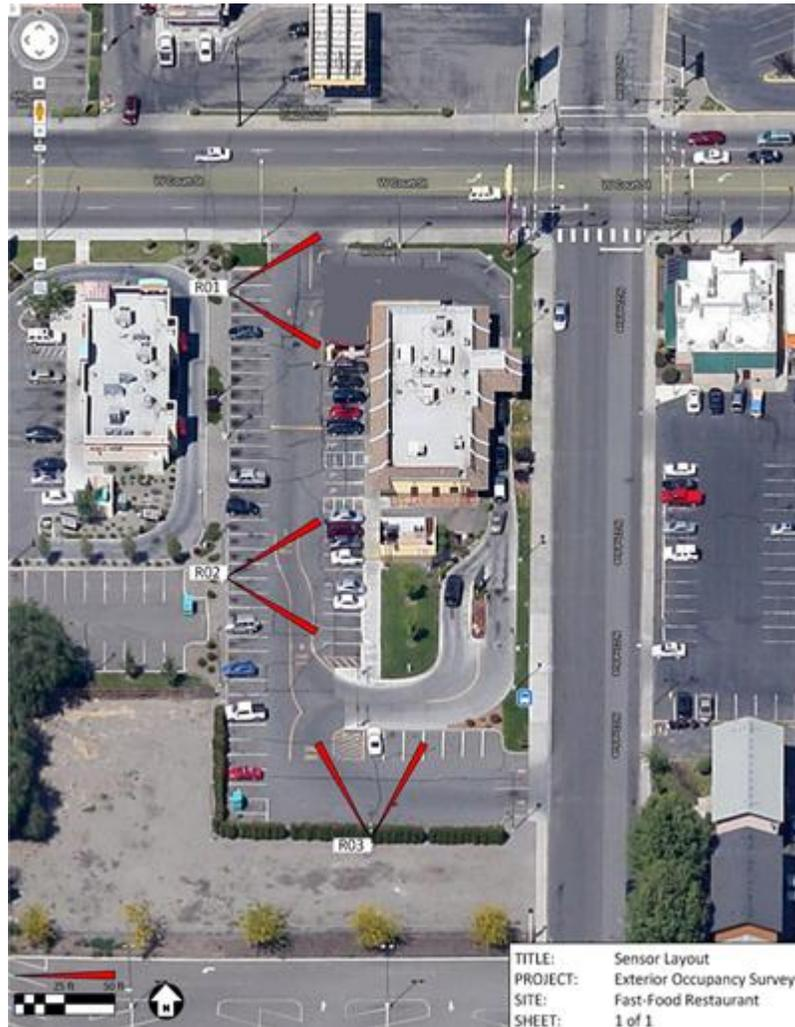
**FIGURE 19: SENSOR LAYOUT AT FAST FOOD RESTAURANT HOST SITE IN SOUTHEAST WASHINGTON. R01–R03 REPRESENT THE LOCATIONS OF THE THREE RECEIVERS USED AT THIS SITE. THE RED TRIANGLES EXTENDING FROM THE RECEIVER LOCATIONS REPRESENT INDIVIDUAL SENSORS AND THEIR ORIENTATION.**
