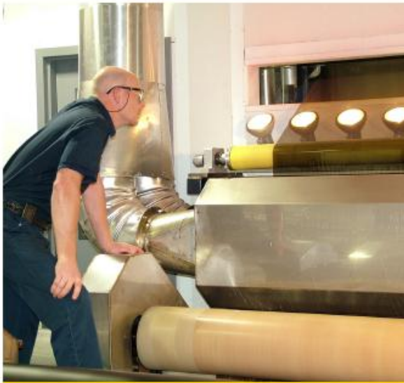
High performance surface-applied film in production being inspected for defects. Note the series of lamps that help in assessing film quality.
