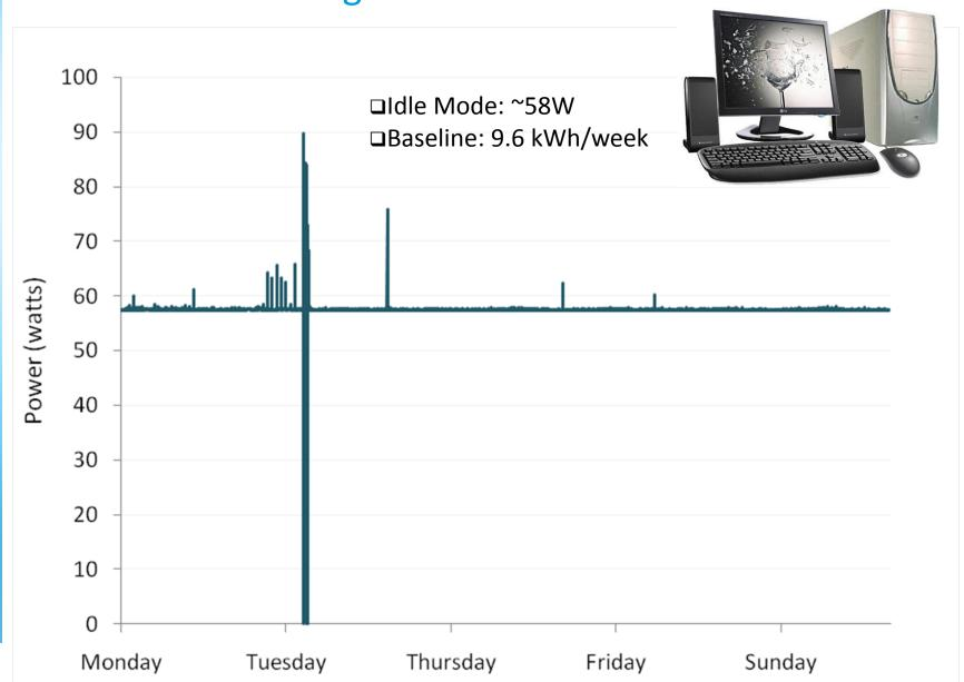
Replaced a Desktop Computer by a Mini-Desktop Computer and Enabled Power Management
