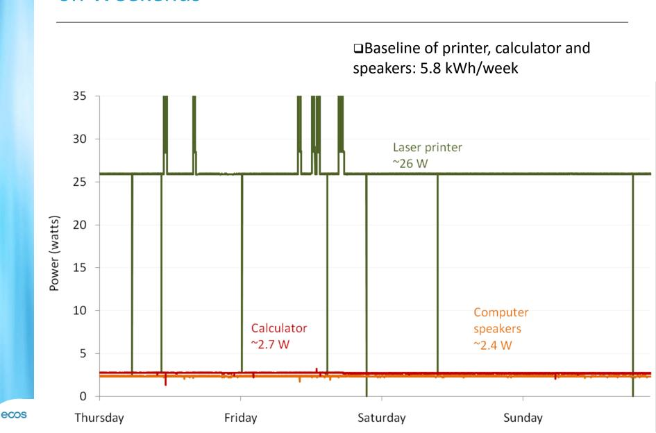
Installed a Timer Plug Strip to Turn Off the Printer, Calculator and Computer Speakers from 9 p.m. to 6 a.m. on Week Days and all Day on Weekends
