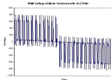
*Voltage at motor terminals after TCI KLC long lead (dV/dT) filter installed.*
