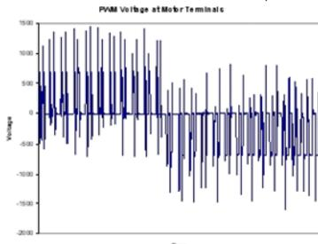
*Long motor leads on a VFD produce damaging voltages at the motor.*
