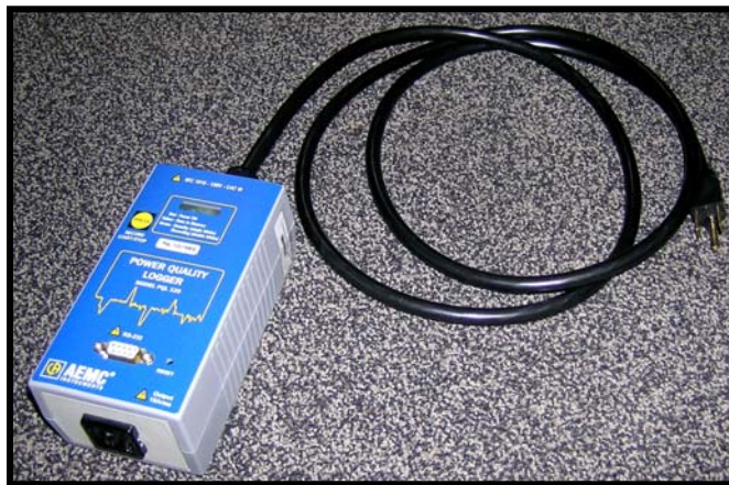
FIGURE 4. POWER QUALITY LOGGER
