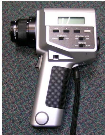
FIGURE 5. CHROMA METER. THE CHROMA METER MEASURES COLOR AND LUMINANCE.
