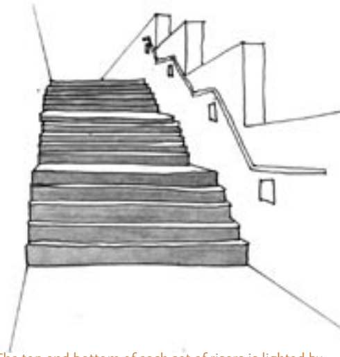
The top and bottom of each set of risers is lit by step-lights recessed into the wall at landings.
