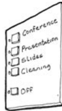
Remote control panel for four-scene pre-set control system
