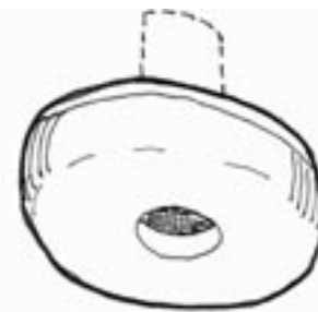
Photosensor placement is a critical decision for daylight harvesting. (They are about 2" in diameter).
