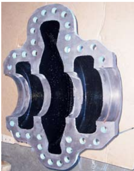
Figure 10 – Denise No. 2 horizontal split-case pump – upper half of pump housing after the application of RILSAN® Fine Powder.
