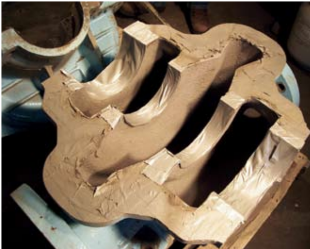
Figure 5. Denise No. 2 horizontal split-case pump – lower half of pump housing after masking the seal areas and grit blast cleaning. A thin dry-film thickness of 0.2 to 0.5-mils (thousandths of an inch) was targeted. After the primer dried about ten minutes, the housing was placed into a convection oven maintained at 525-deg F for one hour. The time and temperature allowed the casting to reach a metal temperature well above the melting point of the RILSAN® Fine Powder grade 625 BLACK MAC ES (melting point of polyamide-11 is 367-deg F).
