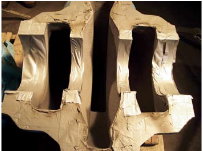
Figure 6. Denise No. 2 horizontal split-case pump – upper half of pump housing after masking the seal areas and grit blast cleaning. solidified into a durable finish. Photos of the coated housings are shown in Figures 9 and 10.
