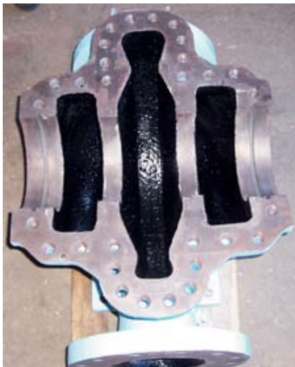
Figure 9. Denise No. 2 horizontal split-case pump – lower half of pump housing after the application of RILSAN® Fine Powder.
