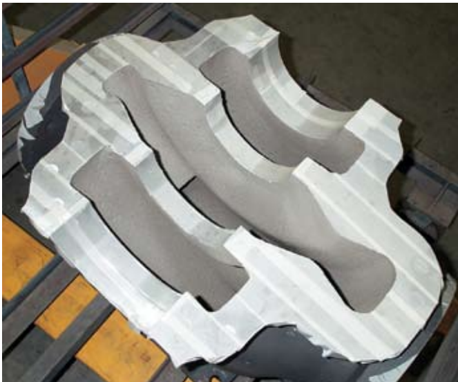
Figure 7. Denise No. 2 horizontal split-case pump – lower half of pump housing after stainless steel plasma coating.
