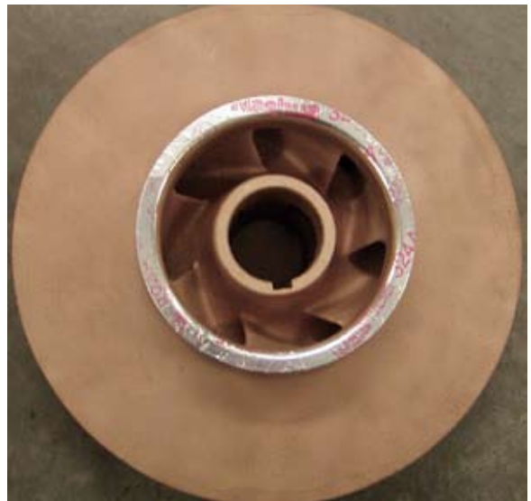
Figure 12 -Denise No. 2 impeller prior to the coating process.
