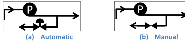
Figure 8: Bypass System Types
