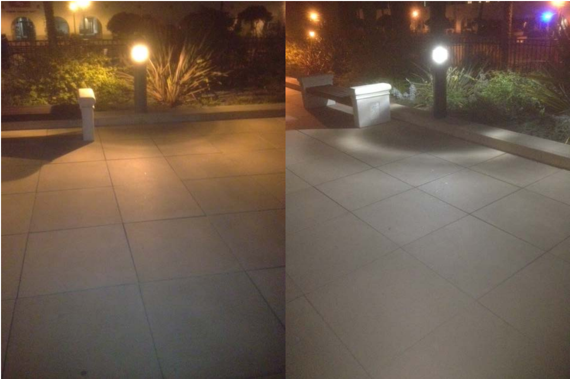
Figure 1: The base case HID (left) and LED solution (right).
