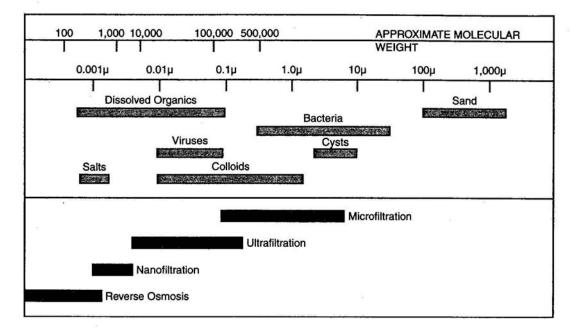
Figure 4.1. Mass Transport in Membrane Filtration
