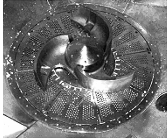
Figure 1. Energy-saving repulper rotor blade
