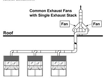
Figure 1. Simple centralized exhaust system.
